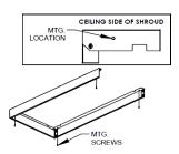
Step 3: Take note of mounting location dimensions, and mark locations on the ceiling as desired. Using approved hardware, secure the 3 pc shroud assy to the ceiling by the mounting locations as shown.
