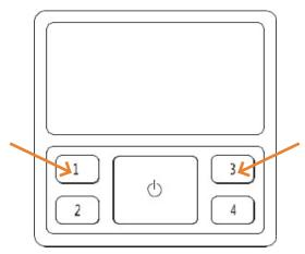
Pressing button 1 and 3 together over 2 seconds achieves reset function and enters pairing mode for 30 seconds. Then, switch can be added by APP searching within 30 seconds.
