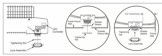
Fixture's wall thickness must be ≤ 0.125" for optimal sensor mounting security.
