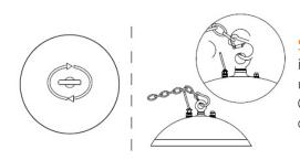
Step 1: Insert the o-hook into lamp body and screw up by rotating clockwise. Connect the carabiner with o-hook.
