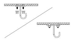
Step 3: Fix the suspension parts onto ceiling surface and tighten the screws.
