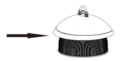
Fix the reflector on the lamp body.
