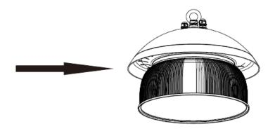
Fix the connecting plate on the lamp body with screws, then fasten reflector on the connecting plate.
