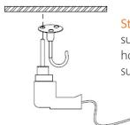
Step 2: Drill in ceiling surface according to the hole location of suspension parts.
