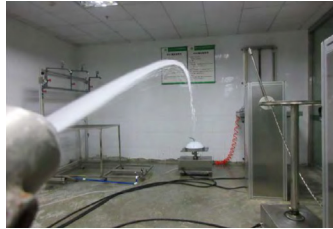
The FRHBN has been tested to meet stringent IP69K high pressure, high temperature washdown requirements
