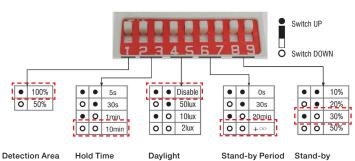
Detection Area H In this area, movement will be detected and able to trigger the sensor. 100% detection area is also known as strong sensitvity.
