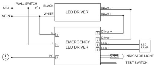
This wiring diagram is suitable for LED lamps with power less than 120W and the output current of the lamp's driver does not exceed 3A
