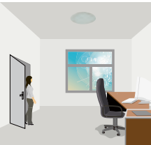
With sufficient natural light, the light does not switch on when motion is detected.
