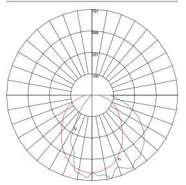
Axial Candela Maximum Candela = 781.15  $Located\ At\ Horizontal\ Angle=0,\ Vertical\ Angle=13.0$  FSWP-SNC-20W
